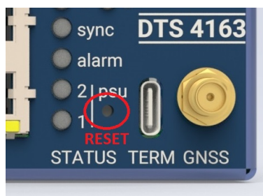
Figure 6: Reset of DTS 4163
