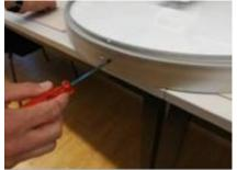
5. try to spread the ring, until the movement and with the complete dial can be removed to the top. The ring is quite strong, so it needs some strength to spread it.
