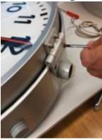
Module without hinge: Remove 4 screws from inside of the clock
