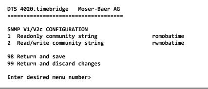
Path: 2 Configuration → 8 SNMP → 5 SNMP V1/V2c security configuration
