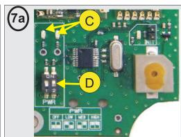
You can adapt the transmission power with two DIP switches (D). LEDs (C) allow you to check your setting.
