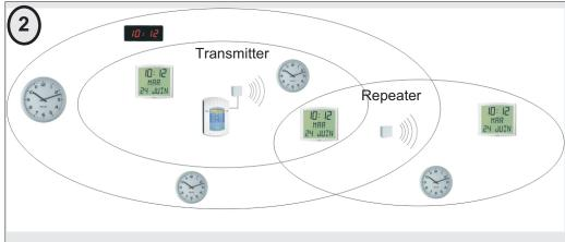
The DHF repeater V2 (ref.: 927241) enables to extend an area non covered by the main DHF transmitter.
