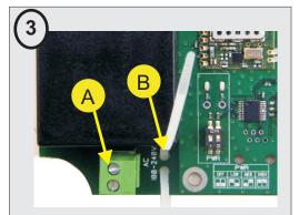
Connect the 230V (A) and secure the powercable with the tie-wrap (B). Apply the power.
