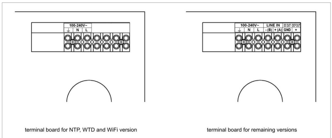
Note: For PoE version is Ethernet cable plugged directly into the connector on the control board (this version is without terminal block)
