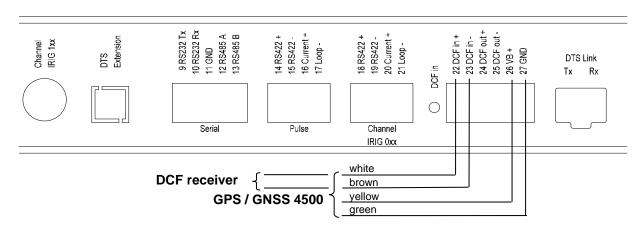
GNSS 3000 according to manual Bx-800813 chap. 9.2 Connection schematics DCF current loop
